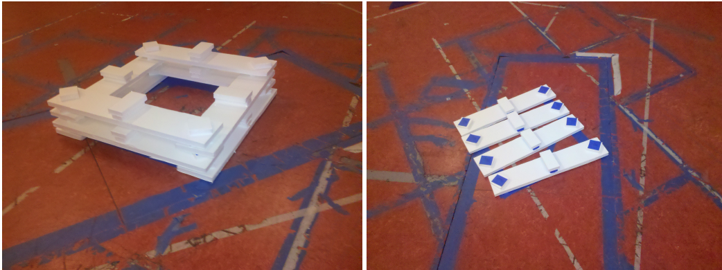
Figure 6-1: The “box” and “wall” shapes built in our experiments. “box” tests the ordering based on physical dependencies, “wall” tests maintenance of reachability.
