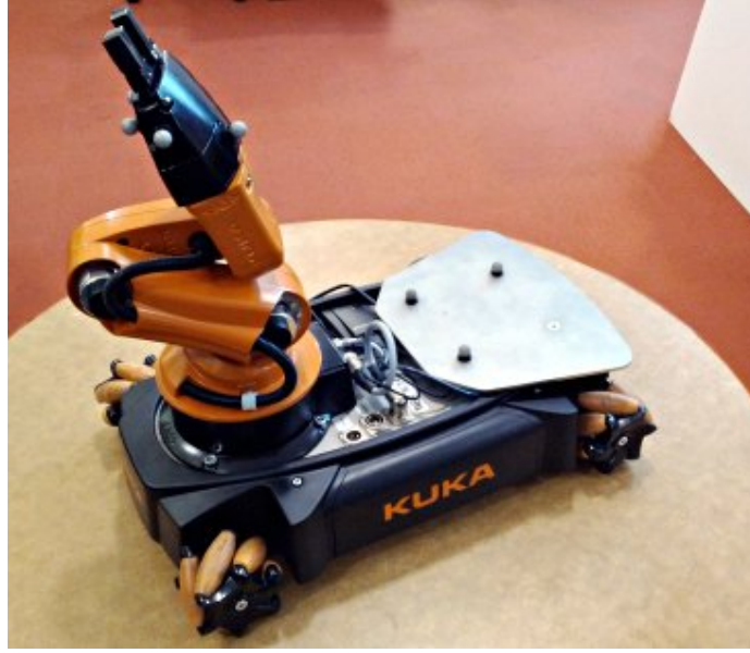
Figure 7-1: Side view of the KUKA YouBot. The holonomic base allows for omnidirectional movement, while the five d.o.f. arm provides high-fidelity manipulation in the workspace around the robot
